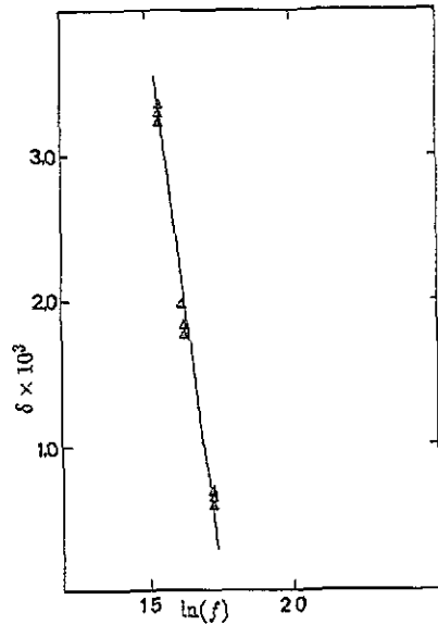
Figure 10. The relation between the Bordoni peak height and the frequency of measurement.
